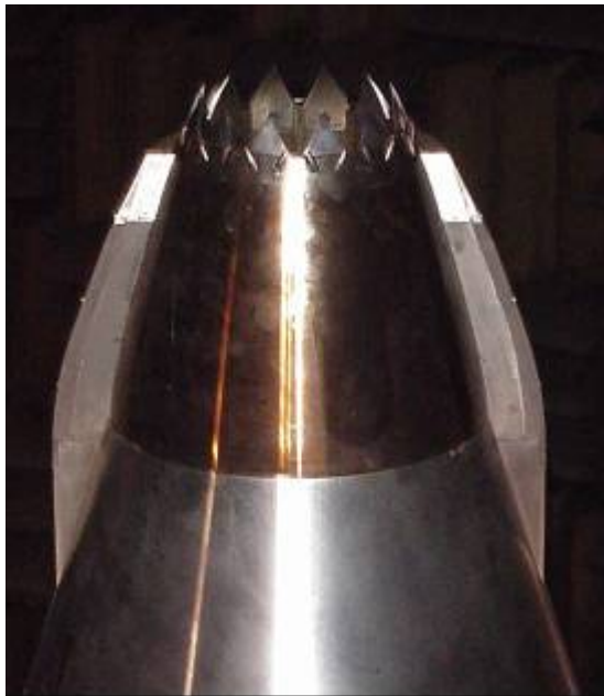
Figure 13 Photograph of C-D chevron nozzle with shield on backside of the nozzle.
