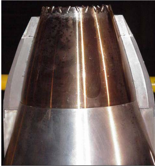
Figure 9. Photograph of scale model C-D nozzle with fluidic chevrons and a fluid shield.
